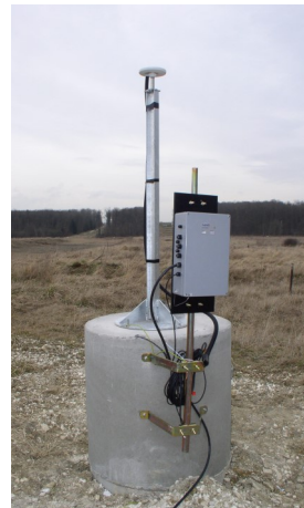
Autonomous SYT GEO RTK-GPS station with high sampling frequency and radio transmission offered a very high quality time series of the 4 meters vertical subsidence recorded during the last two days with an accuracy close to 1 cm.
