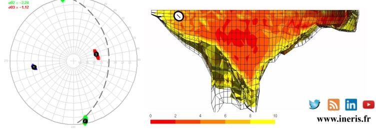
Left : principal stresses computed and projected on a lower hemisphere. Uncertainty is graphically represented as centered colored stains. Gray-dotted line shows the estimated orientation of the rock foundation below zone 1. Right : 3D elevation view of the dam with the major principal stress  $\sigma_1$  contours mapped on its downstream face. Modelling by EdF-CIH.
