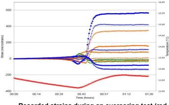
Recorded strains during an overcoring test (red curve shows the temperature).
