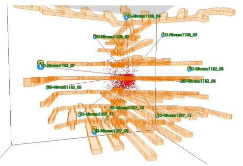
3D perspective of a 300x300x300m mine layout and its local seismic network, showing ray tracing, source location and density probability function related to a significant event.
