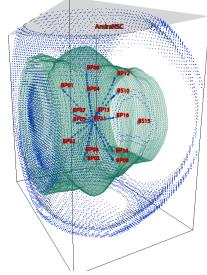
3D perspective of an acoustic array encased in an engineered concrete bulkhead to seal a deep tunnel.
