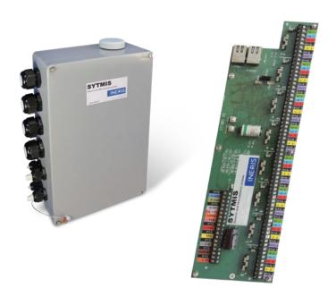
**Ineris** provides monitoring services based on the SYTMIS<sup>®</sup> equipment series as a unique range of systems designed for real-time acoustic and seismic monitoring in a wide range of industrial applications.
