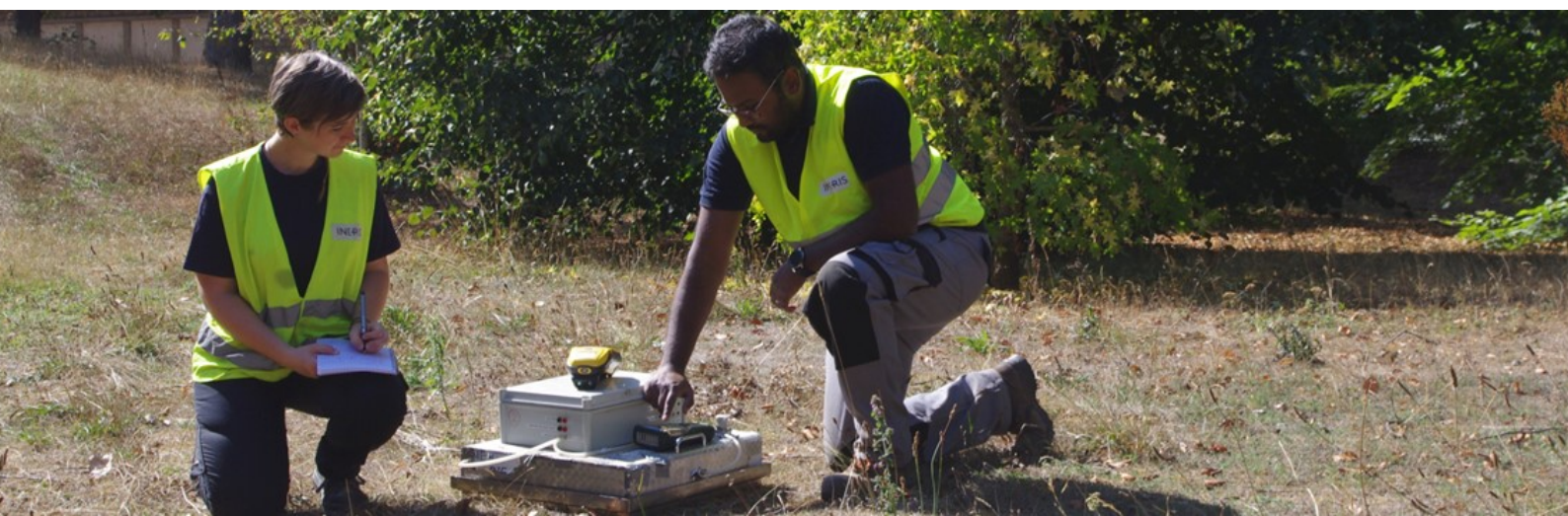
Surface gas flux measurement using the accumulation chamber developed and patented by Ineris.
