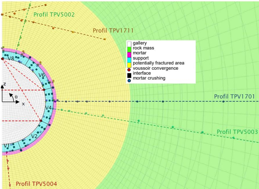
Representation of the virtual sensors positioned within the numerical model
