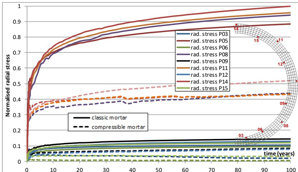
Time history of radial stresses within the arched segments with classic mortar (solid lines) and compressible mortar (dotted lines): the compressible material reduces the amount of radial compression transmitted to the concrete in the arched segment.
