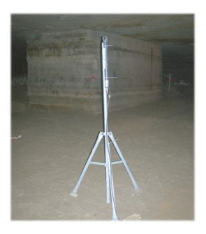
Built with high standard metrological characteristics, the probe has an easy-to-handle rugged housing for fast installation in large underground junctions or in naturally protecting recesses. It features easy recovery and removal along with minimal maintenance thanks to its long term stability and integrated autotest functionality.
